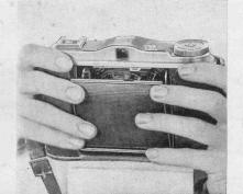
To lock camera front, press front firmly against camera body until it locks into the closed position.
