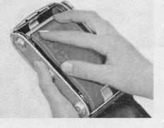
To thread film, tear adhesive tape, carefully remove free ends of tape; then unfold flap of backing paper and thread paper into wide opening of spool slot.
