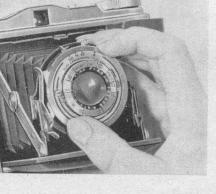
To set the shutter speed, turn milled shutter ring until "V" mark registers with desired shutter speed (25 — 75-200, i. e.,  $\frac{1}{25}-\frac{1}{75}-\frac{1}{200}$  second).
