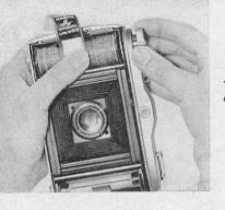
To unload film spool, open camera back (see p. 4), pull out winding knob, at the same time turning it clockwise.
