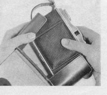
To load camera, unscrew dummy tripod screw at bottom of ever-ready case, take camera out.
