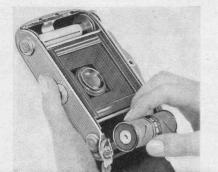
To insert new spool, slip slotted spool end over fixed carrier peg, return hinged carrier to engage second peg, swing spool into chamber.
