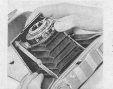
To set the diaphragm, place right thumb on stop lever and set at desired mark (4,5-5,6-8-11-16-22-32).
