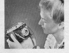
Before every exposure check settings of diaphragm, shutter speed, distance,
