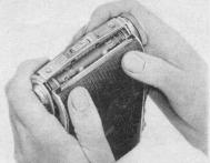
To open camera front, press buttom on top of camera and the lens board will spring forward; if necessary, assist the braces to snap into position.
