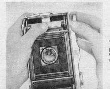
To position empty spool, push spool into chamber, gently push in winding knob while rotating it clockwise until winder key has engaged slotted spool end.
